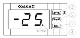
**1 - Key Set** : It is used to program the Set Point and the functionning parameters.
