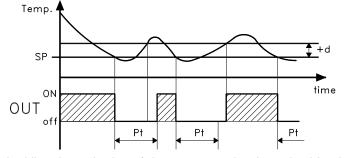
Avoiding the activation of the output can be determined by the switch on delay mode.
