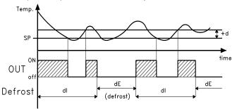
When defrost cycle is in process, "dF" is being displayed. With the par. "dL", it is possible to use the display during defrost. The equipment can display "dF" in alternation with the temperature measured by the probe (dL = oF) or only "dF" (dL = Lb).
