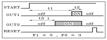
Received the start signal the instrument begins the counting and exactly operating on the output OUT 2 in the same way with which it operates the function F1 on the output OUT1.
