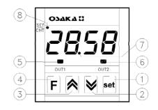
1 - Key Set : Used for the set point setting and to program the functioning parameters
